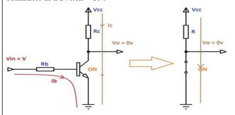
Transistor as a Switch ON
