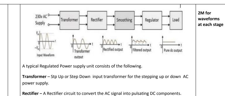
**Smoothing** – A filtering circuit to smoothen the variations present in the rectified output.
