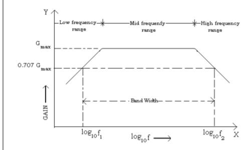
Bandwidth of the amplifier = Higher frequency - Lower frequency
